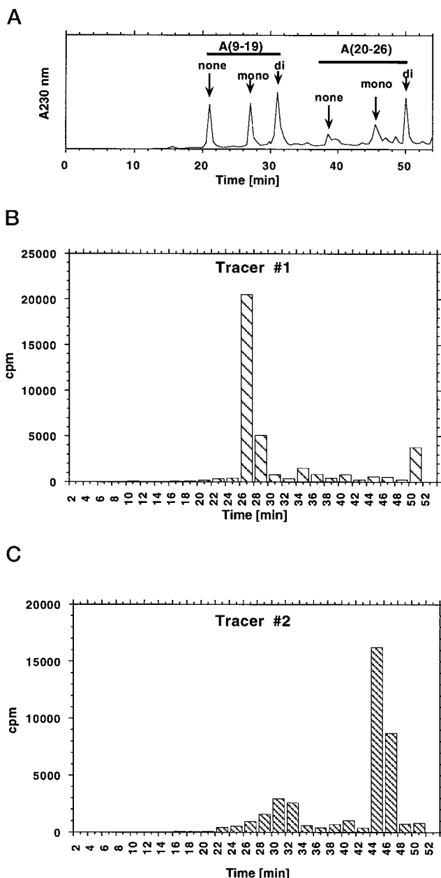
FIG. 4. HPLC separation of a tracer V8/trypsin digest followed by reduction. A , the reaction was spiked with partially iodinated reduced peptides of the sequence A(9–19) and A(20–26) on Aquapore 300 (2.1 × 30 mm). The mobile phase was 0.1% trifluoroacetic acid in water (A) and 0.1% trifluoroacetic acid in 80% acetonitrile. Separation was achieved by running a 1-h linear gradient from 5 to 50% B; the effluent was monitored by UV absorbance at 230 nm. B , digest of tracer #1. Fractions of 2 min were manually collected and counted in a \gamma counter. The majority of the counts were eluted in the position of mono-iodinated peptide A(9–19), indicating that tracer #1 is ^{125}\text{I} -Tyr(A9) human RLF. C , digest of tracer #2. Fractions of 2 min were
